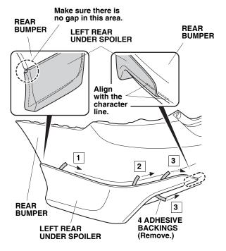
12. Remove the four adhesive backings in the order shown. Press the left rear under spoiler firmly against the rear bumper with the palms of your hands to set the adhesive.  Tighten the two female clips loosely installed in step 10.
