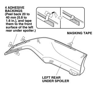
9. Install the left rear under spoiler with one bumper clip.
